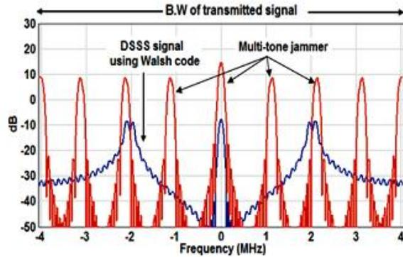
Fig.(11): Frequency spectrum of the Transmitted Signal under the effect of MTJ for  $J/S=10\text{dB}$  using Walsh code.
