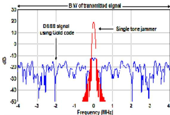
Fig.6:Frequency spectrum of the transmitted signal under the effect of STJ for J/S=10dB using Gold code
