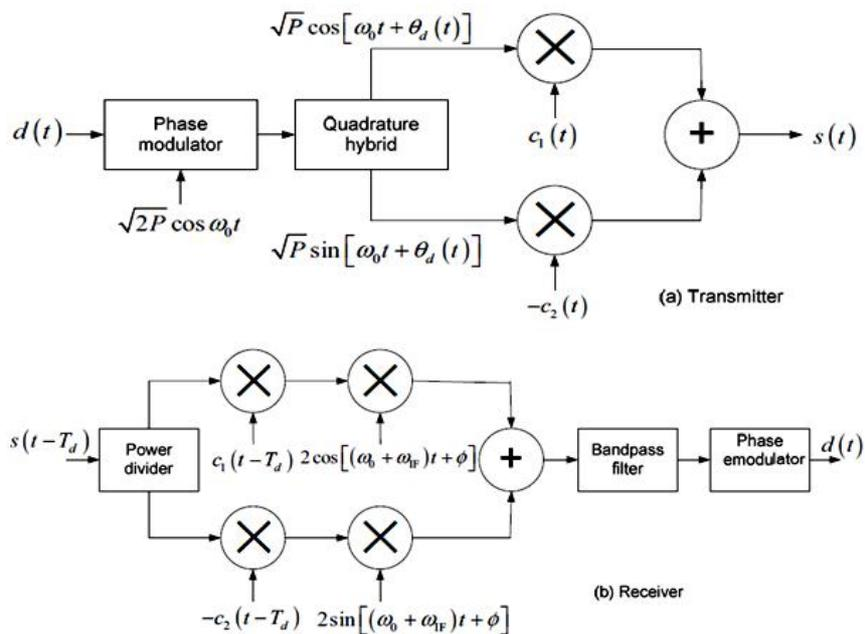
**Fig.1: Block diagrams of : (a) transmitter and (b) receiver for QPSK spreading with arbitrary phase modulation.**
