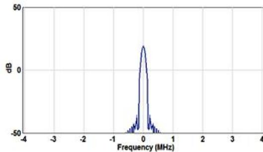
**Fig.(12): Autocorrelation function of Gold code.**
