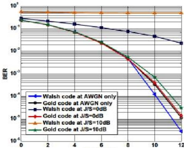
Fig.4: Comparison BER for DSSS in presence of STJ .
