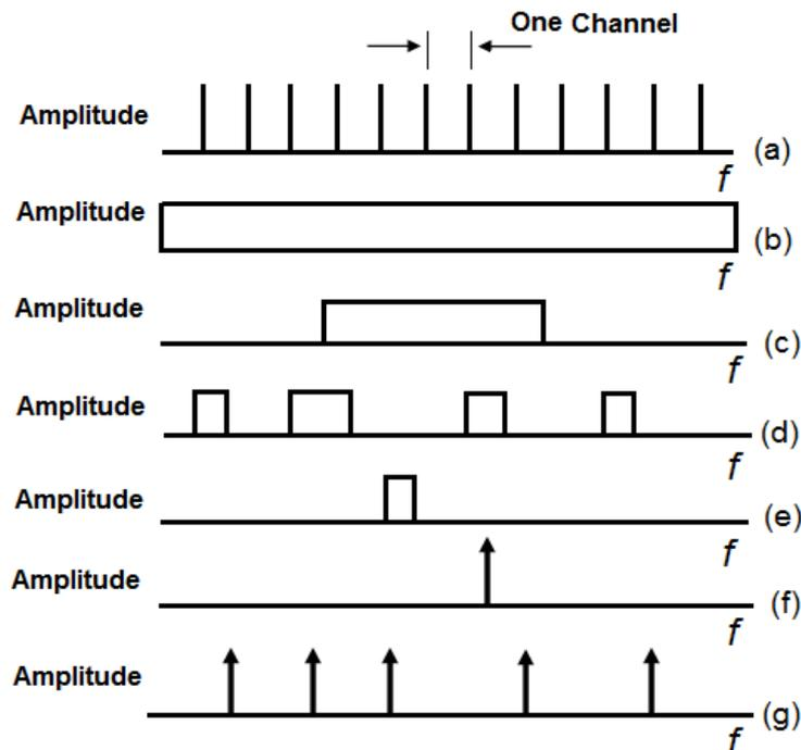
**Fig.2: Possible strategies a jammer may use based on the channelized spectrum shown in (a) and (b) Broad-band jamming (BBN), (c) contiguous partial-band jamming (PBN),(d) noncontiguous partial band jamming (PBN), (e) narrow band noise jamming (NBN), (f) single-tone (ST) jamming, and (g) multi tone (MT) jamming**
