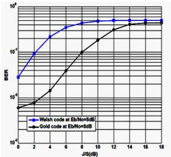
Fig.9: Comparison BER for presence of MTJ for different Values of J/S ratio.
