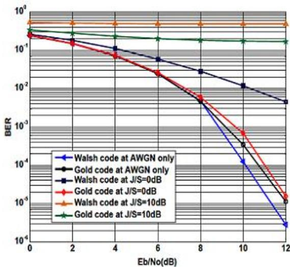
Fig.8: Comparison BER for DSSS in DSSS in Presence of MTJ.
