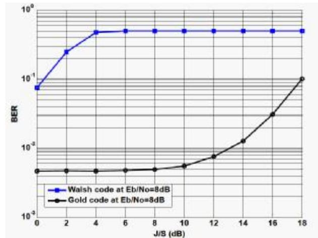
Fig.5: Comparison BER for DSSS in presence of STJ for different value of J/S ratio
