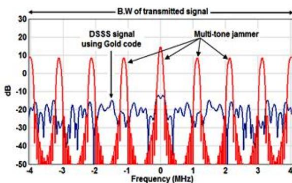
Fig.(10): Frequency spectrum of the Transmitted signal under the effect of MTJ for  $J/S=10\text{dB}$  using Gold code.
