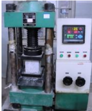
Plate (4) Digital compression machine used for cube concrete compressive strength test.
