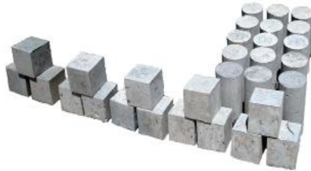
Plate (2) Total control specimens (15 cylinders and 15 cubes).
