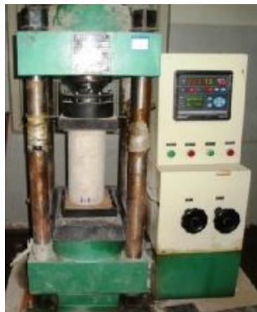
Plate (3) Digital compression machine used for cylinder concrete compressive strength test.
