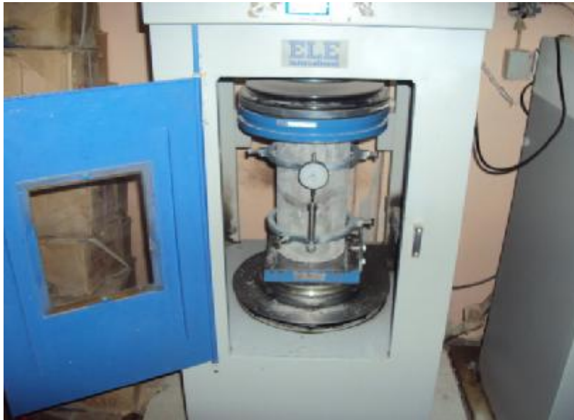
Figure (1) Cylinder Compressive strength and Compressometer with dial gauge.
