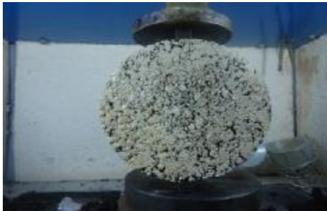
Plo(7) Resilient modules setup test.
