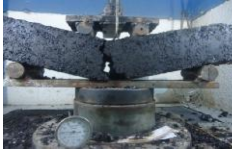
Plot (5) Beam failure .
