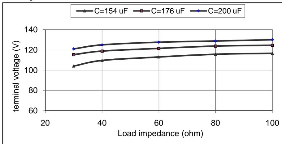
**Fig. (5): Terminal voltage variation against load impedance at different values of excitation capacitance.**
