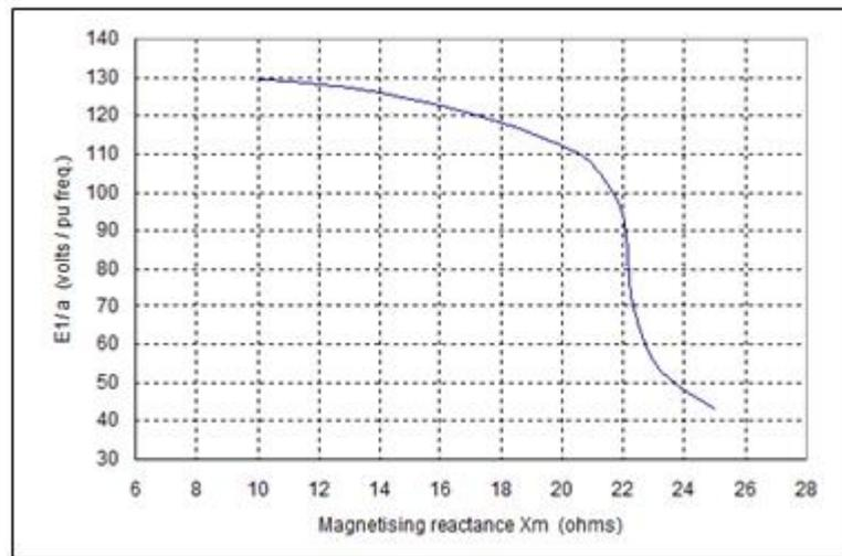
**Fig. (2) Variation of normalized air gap voltage ( $E_1/a$ ) with magnetizing reactance ( $X_m$ )**
