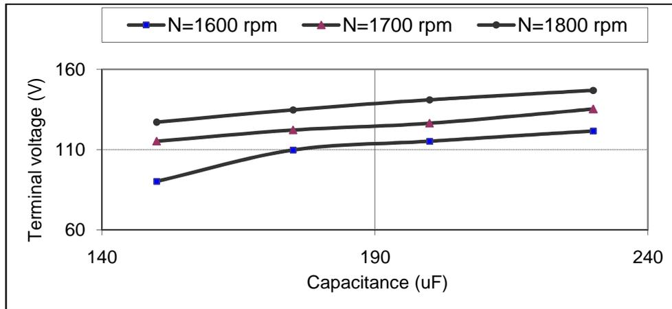
**Fig. (4) Terminal voltage variation versus excitation capacitance at different rotor speeds**
