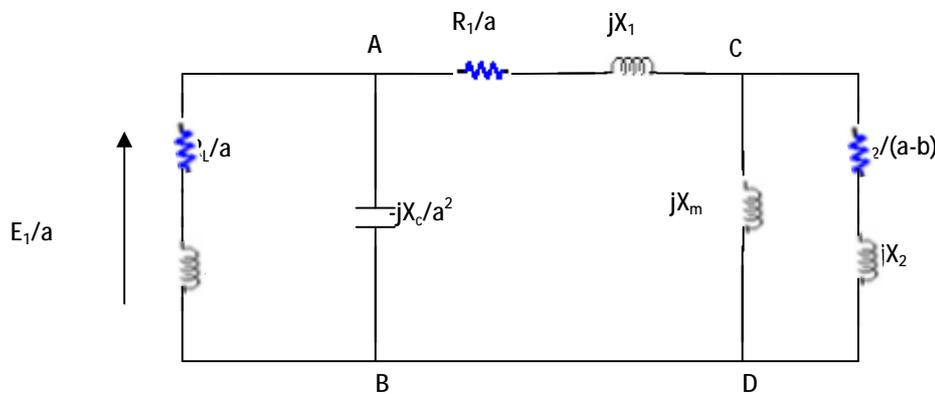
**Fig. (1) Per-phase equivalent circuit of self-excited induction generator**
