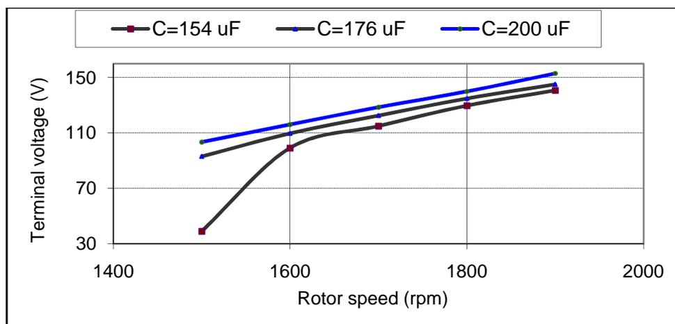
**Fig. (3) Terminal voltage variation against rotor speed at different excitation capacitances**
