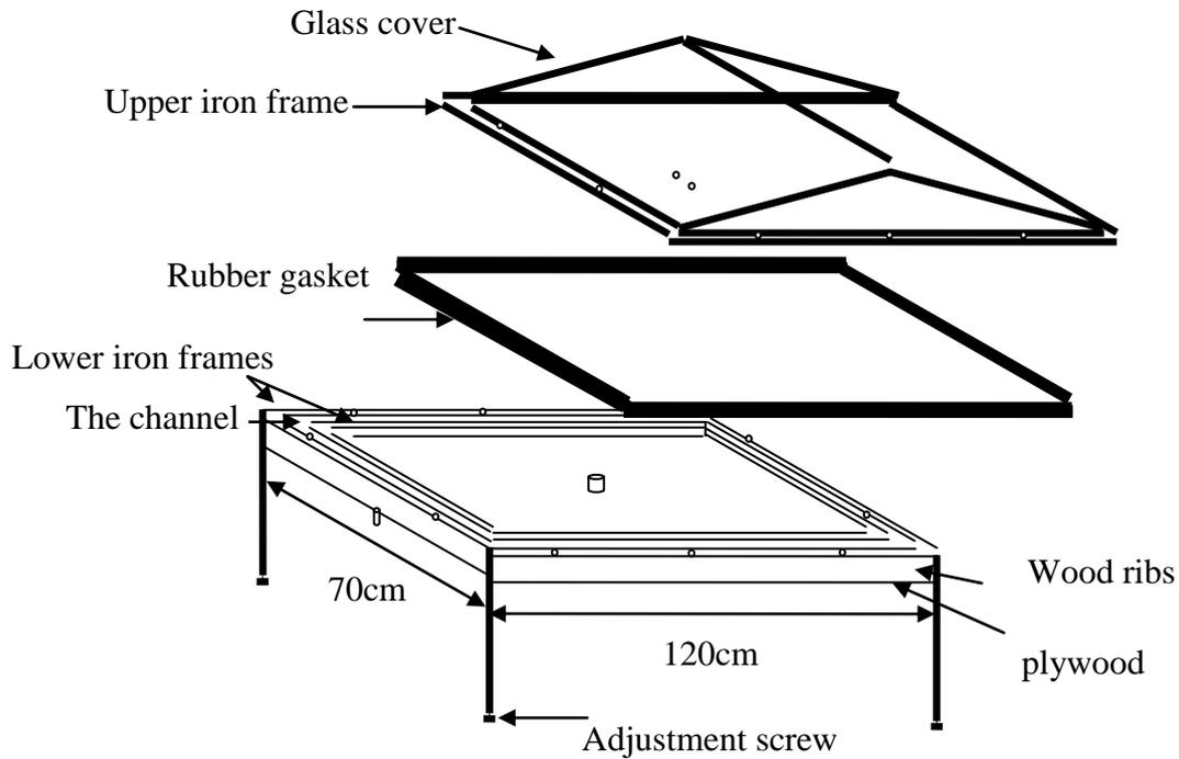
**Fig.(1): Schematic diagram of the solar still**
