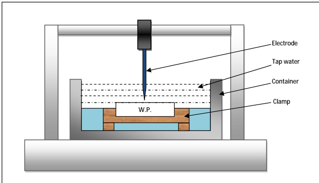
Figure (1) The schematic diagram of the experiment setup.
