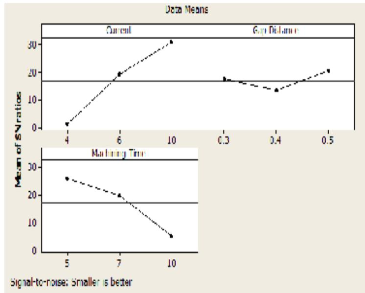
Figure (4) Main effects plot for S/N ratios for overcut.
