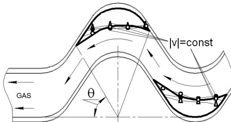
**Figure.4.** Geometrical zones of the filtering sections in the separation channel of the louver inertial filtering gas separator disposition. ( $Re \geq 10000$ ).
