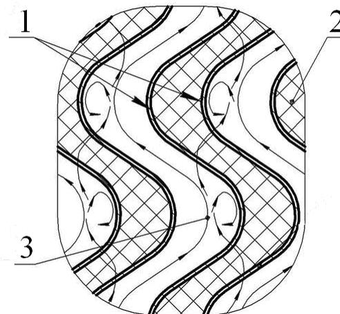
**Figure 6.** the gas fluid movement along the separation board of the IF drop catcher scheme:
