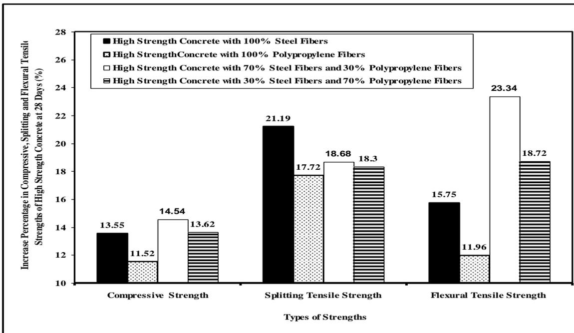
Fig.4 Increase Percentages in Compressive, Splitting and Flexural Tensile Strengths of High Strength Concrete at 28 Days (%)
