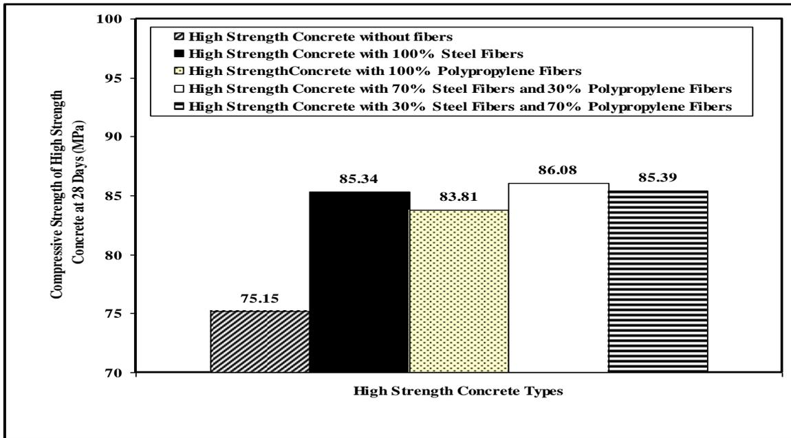
Fig. 1 The Effect of Fiber Types and Hybrid Fibers on the Compressive Strength of High Strength Concrete
