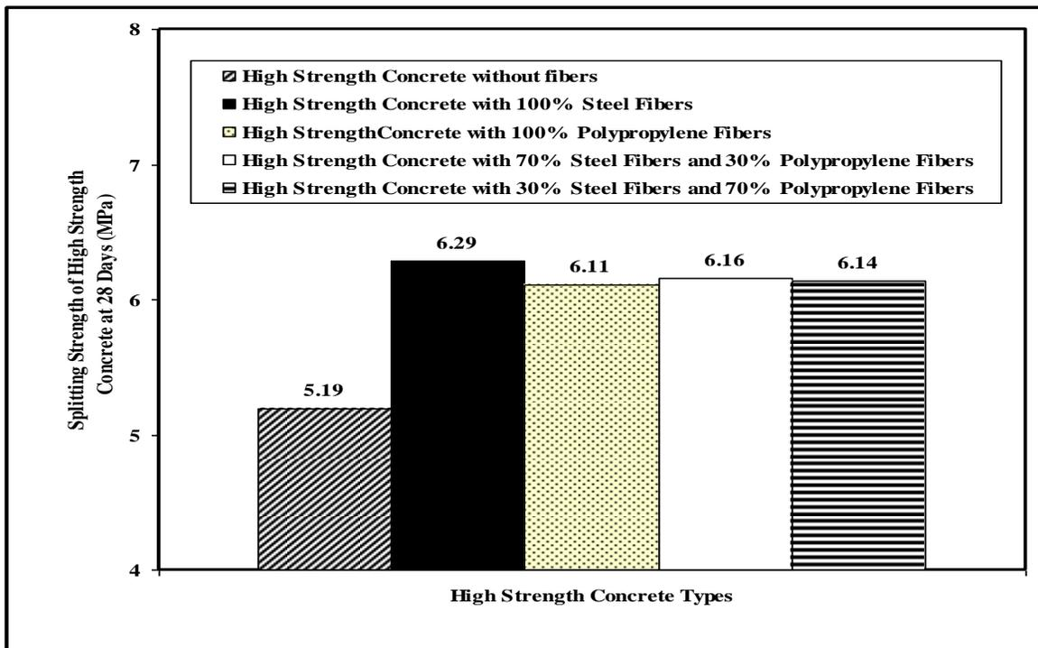
Fig. 2 The Effect of Fiber Types and Hybrid Fibers on the Splitting Strength of High Strength Concrete
