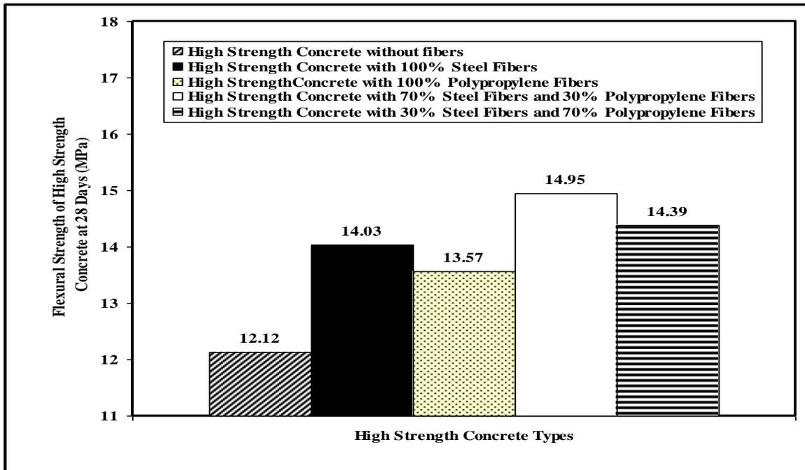
Fig. 3 The Effect of Fiber Types and Hybrid Fibers on the Flexural Strength of High Strength Concrete
