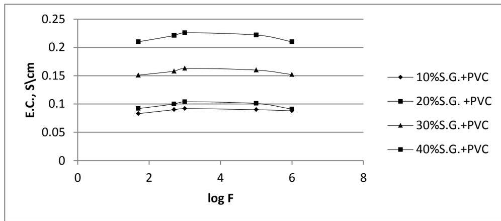
Figure 5: electrical conductivity of synthetic graphite at different frequency
