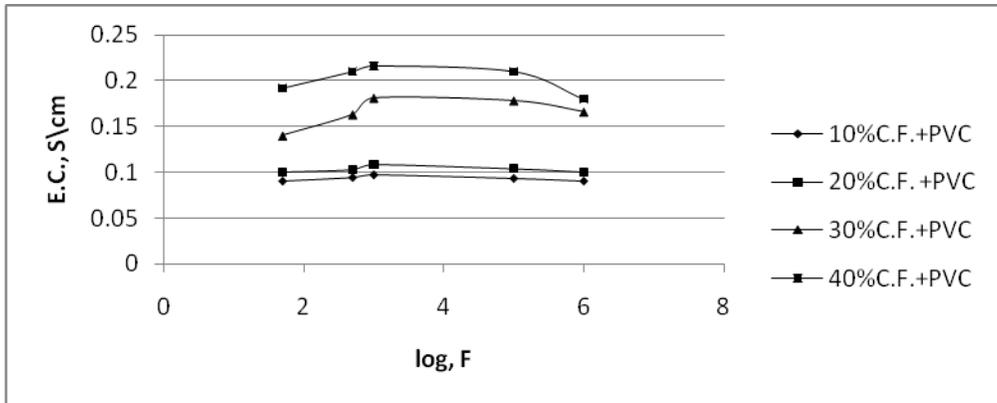
Figure 4: electrical conductivity of carbon fiber at different frequency
