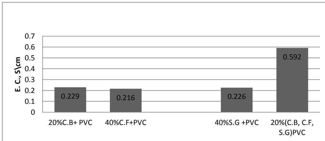
Figure2: Typical electrical conductivity of different fillers reinforced PVC
