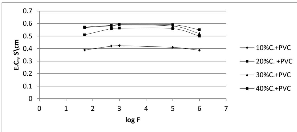
Figure 6: electrical conductivity of composite at different frequency
