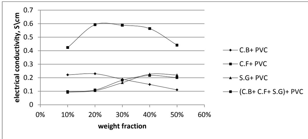
Figure 1: Electrical conductivity of different fillers reinforced PVC
