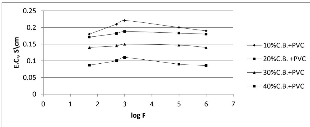
Figure 3: electrical conductivity of carbon black at different frequency
