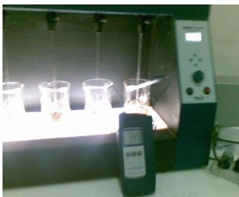
**Fig. (1) Laboratory adsorption unit (Jar Test).**
