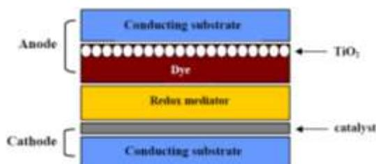
Fig. (2) The components of dye-sensitized solar cell [6]
