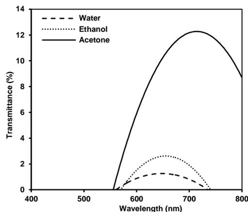
Fig. (4) Averaged transmittance spectra of the *Hibiscus sabdariffa* organic dye solved in different solvents within 400-800nm
