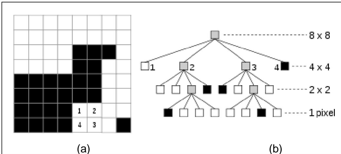
Figure (5) image representation using quad tree. (a) 8 x 8 pixel image . (b) The quad tree representation of the image in (a). The quadrants are shown in clockwise order from the top-left quadrant,[2]
