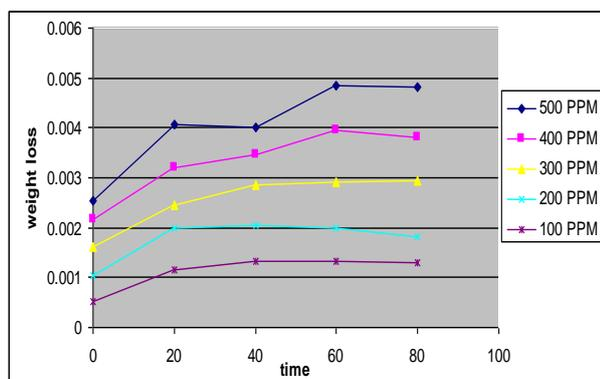
**Fig. (2) Weight loss vs. immersion time for Zn strip in 2M HCl in presence of inhibitor at (500, 400, 300, 200 and 100) ppm of inhibitor.**
