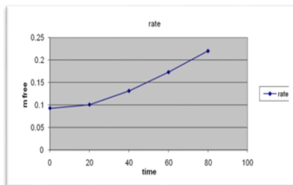
**Fig.(1) Weight loss vs. immersion time for Zn strip in 2M HCl without inhibitor at 25°C.**
