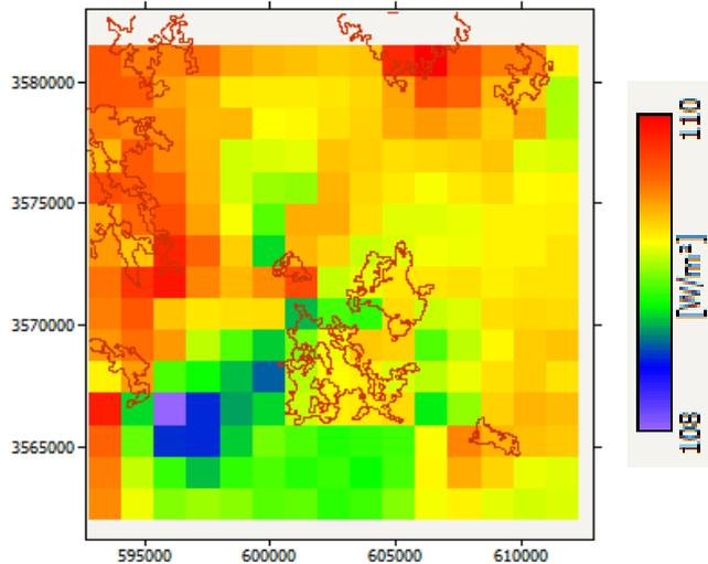
Figure 5-The power density produced by the wind for the 12 sectors.
