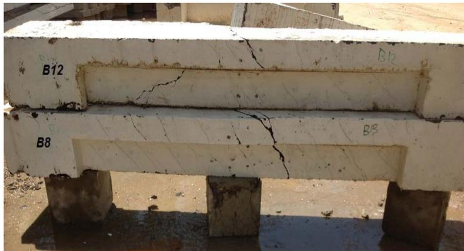
**Fig. (14) : Failure of Group H Specimens**
