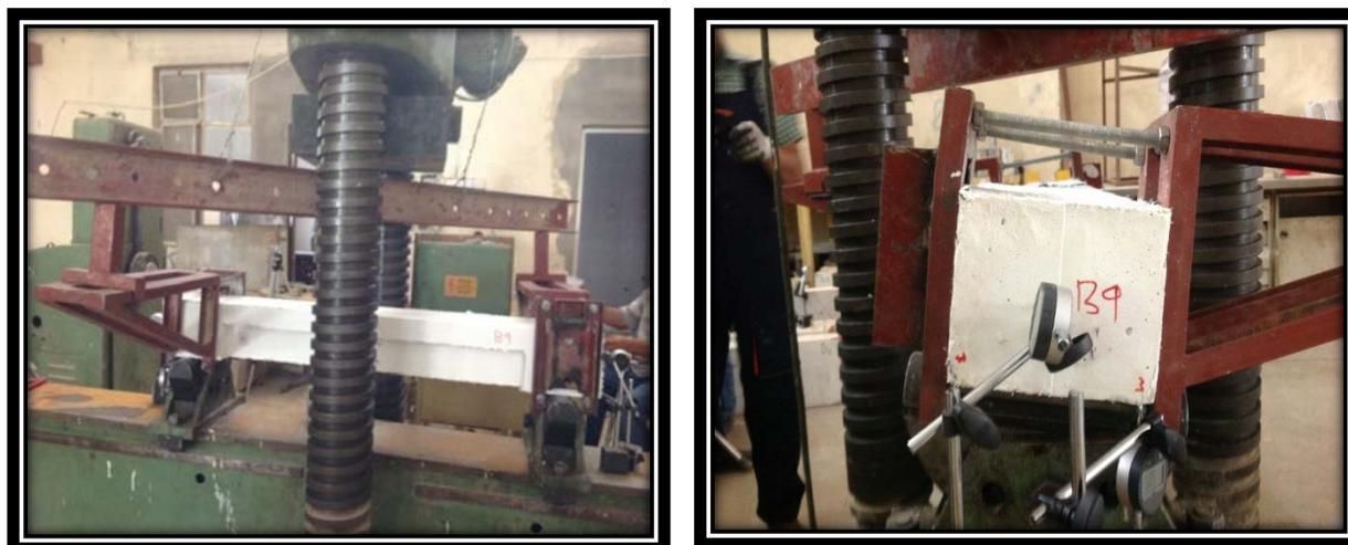
**Fig. (7) Angle of Twist and Elongation Measurement**
