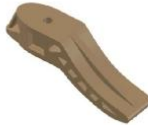
Figure (3) Final Solid Model of KEEL OF SACH Foot.
