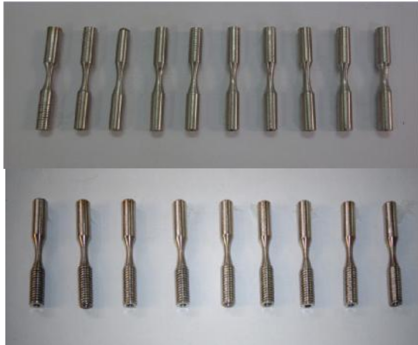
Figure (11) Fatigue specimens before test.
