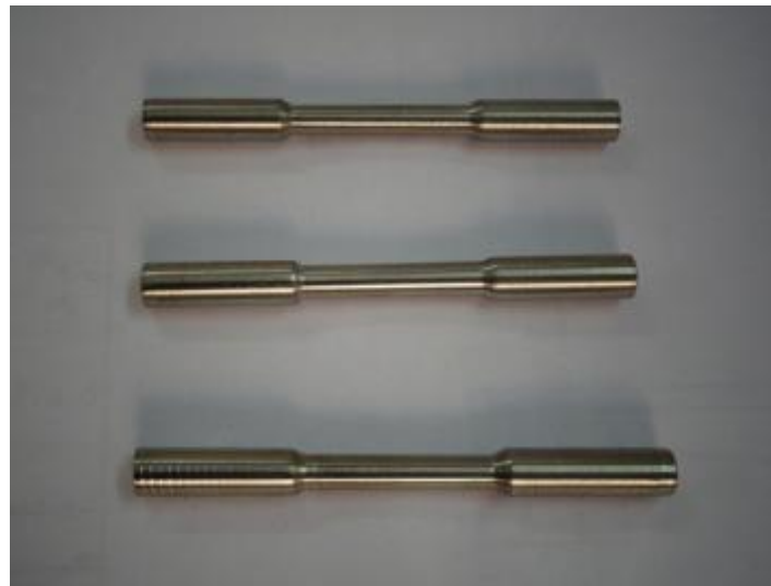
Figure (10) Tensile test specimens before test .
